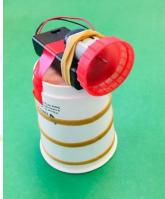
step 8: Choose 4 felt pens and attach them (pointing down) to the sides of the cup by trapping them underneath the elastic bands. Adjust them so they are all level and don't extend above the cup base, where the motor and battery are sitting.
