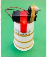
**Step 7:** Use the cocktail stick to make a **very small off-centre** hole in the milk bottle top. Push the milk bottle top onto the part of the motor that spins. Switch on and test again.
