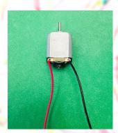
Step 2: Attach the battery holder wires to the motor by bending the exposed metal around the D rings on the motor - one wire to each D ring - it doesn't matter which.
