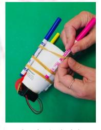
If the motor doesn't spin, check the wires are connected to the D rings.
